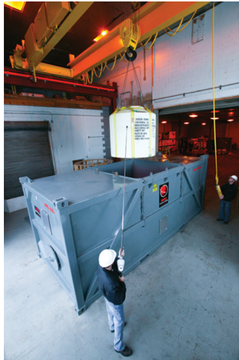
HIC CASK BEING LOWERED INTO A SHIELDED MULTI USE TYPE A CONTAINER
