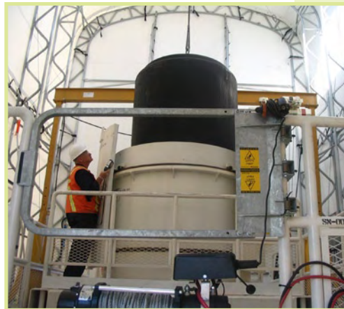
Placing the liners into overpack containers
